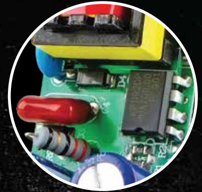
4KV SURGE PROTECTION
