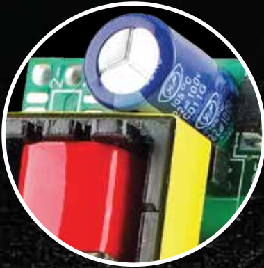
LOW QUALITY CAPACITOR WITH FAKE HOURS PRINTED
